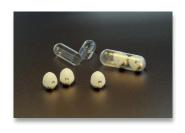
7 February- Engineers have developed a tiny robotic capsule that injects insulin once it lands in the stomach. Once ingested, a tiny device called Soma positions itself against the stomach wall and injects insulin into the bloodstream. Here was the challenge for bioengineers: Find a way for patients to take drugs — like insulin or monoclonal antibodies used to
